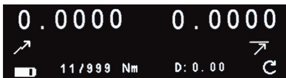
Screen 3 on the third press Click mode with peak value displayed.
