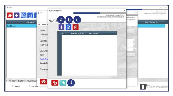
This will only be used if the job is intended for a wrench transducer – the job will then look to make sure an adapter is fitted onto the wrench and matches the details set.
