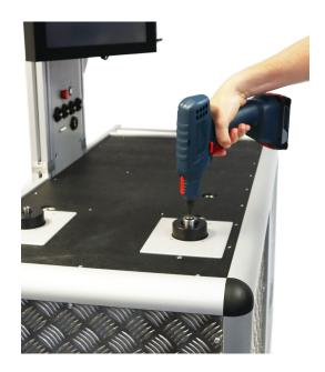
Crane's tJRS joint simulator test bench sets the standard for accurate and precision tool testing and torque management.
