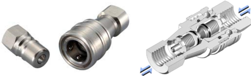
When disconnecting, both socket and plug are sealed by automatic shut off valves instantly. When connecting, automatic shut off valves are open and the socket is sealed by O-ring. Fluid can flow from both socket and plug.
